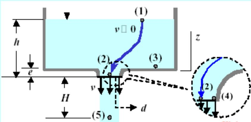
$$z_1 + \frac{p_1}{\gamma} + \frac{v_1^2}{2g} = z_2 + \frac{p_2}{\gamma} + \frac{v_2^2}{2g}$$
