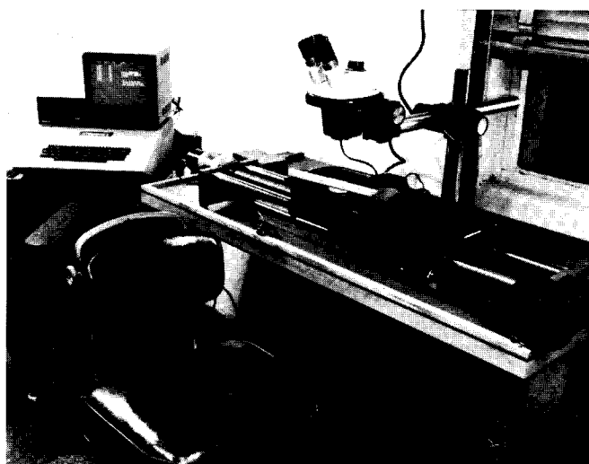
Figure 24—Sliding-stage micrometer/ microcomputer for measuring tree rings.
