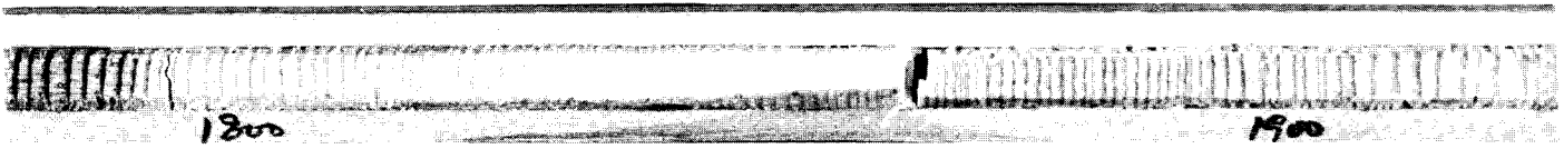
Figure 3 —Mounted, twisted core showing poor alignment of tracheid cells.
