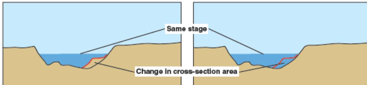
Erosion of part of a channel results in an increased cross-sectional area in the diagram on the right and the potential for conveying a larger quantity of water at the same stage.
