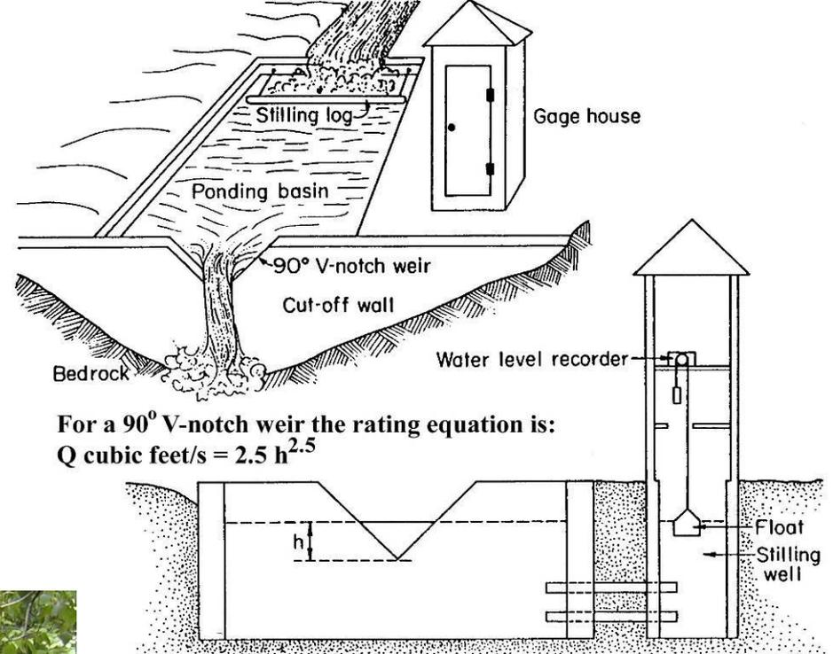
For a 90° V-notch weir the rating equation is:
