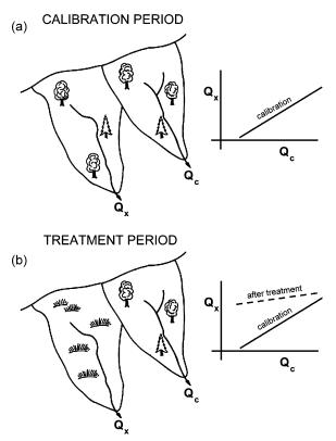
Fig. 1. Sketch of a paired-watershed experiment (from Hewlett, 1982).
