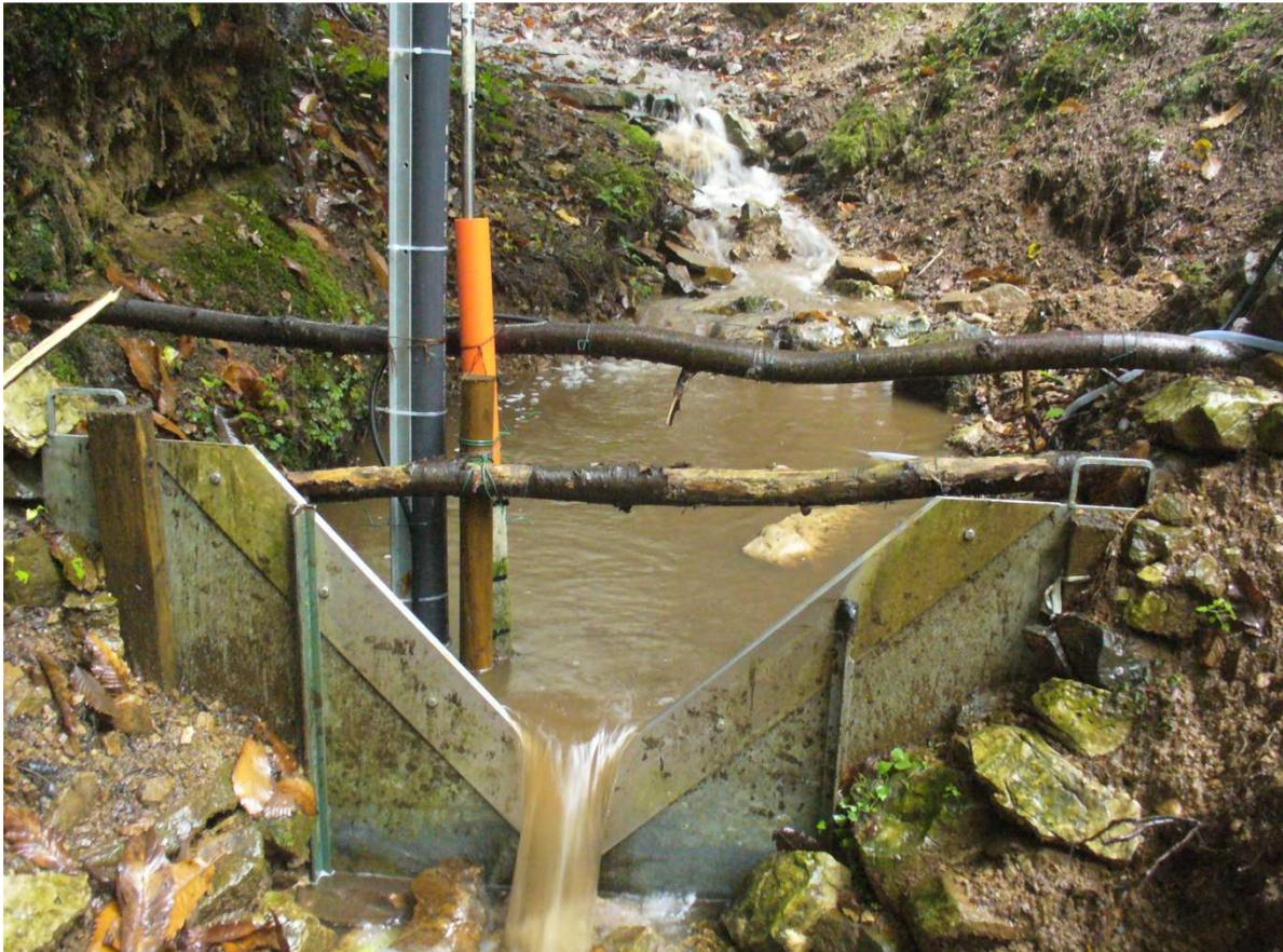
Figure 7. Streamgauge during a rainfall-runoff event.
