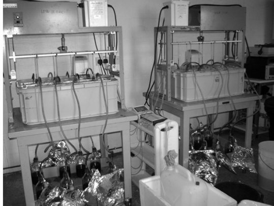
RUSITEC Rumen simulating fermentor (Czerkawski e Breckenridge, 1977)
