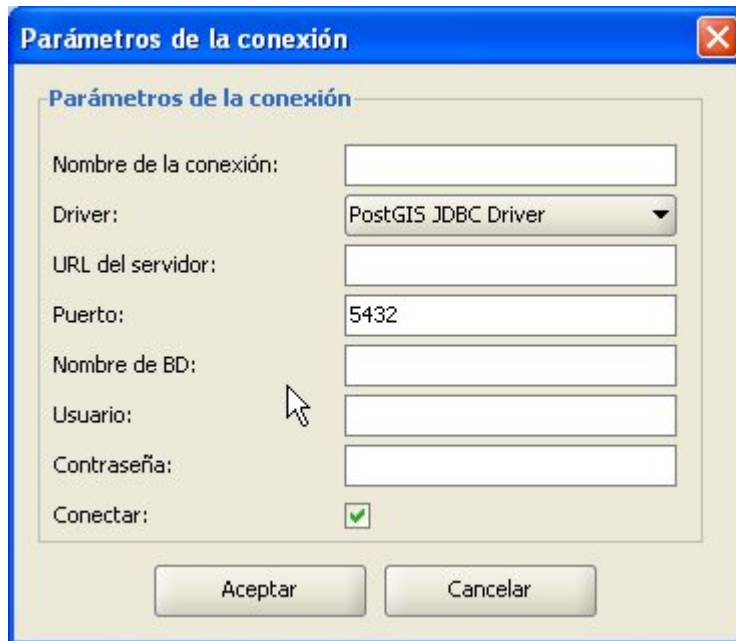
Figure 3. Adding a new connection
