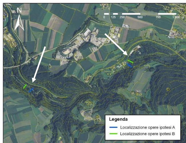
**Fig.11** Arrows indicate the sites identified for the placement of the two structures comprising the trapping system, with two options (A and B) differing slightly in terms of structure size and exact location. Flow is from right to left.
