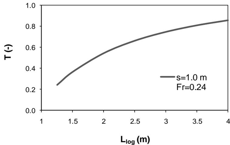
**Fig.13** Variation of trapping efficiency  $T$  as a function of log length for a filter opening of 1 m under the kinetic conditions ( $Fr=0.24$ ) estimated upstream of the inclined-grid check-dam.
