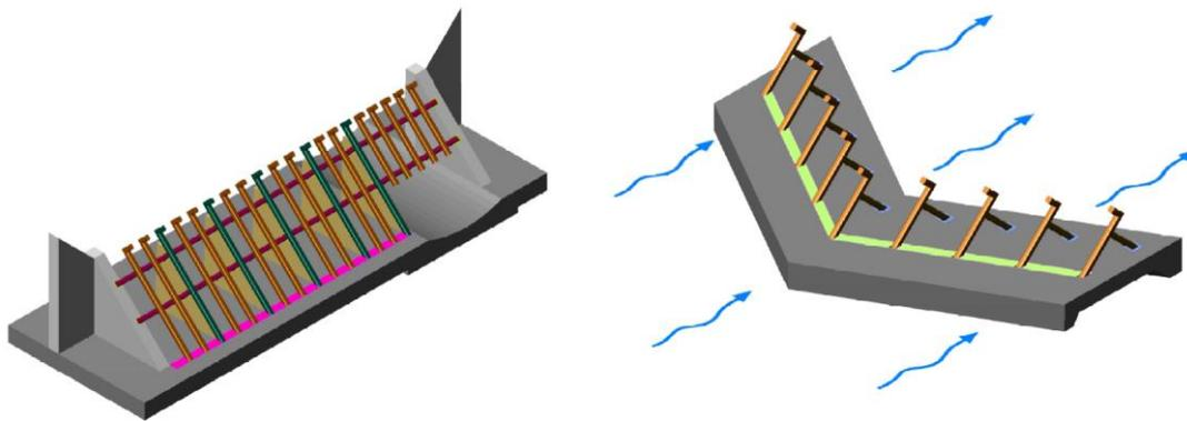
**Fig.12** Three dimensional view of the two wood retention structures: left, the inclined-grid ( $45^\circ$ ) check-dam to be installed upstream; right, the V-shaped inclined ( $45^\circ$ ) racks to be constructed downstream.
