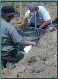
ALWI soil scientists perform double-ring infiltrometer testing in support of a municipal client's spray irrigation project.
