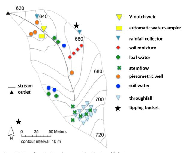
Figure 3. Map of the Ressi catchment and localization of field instruments.
