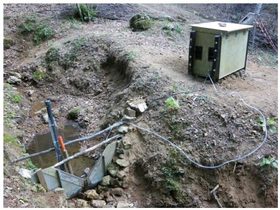
Figure 6. Streamgauge with the box containing the automatic water sampler.
