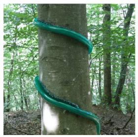
Figure 5. One of the six selected beeches for stemflow measurements.
