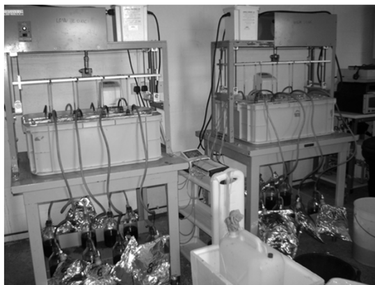
RUSITEC Rumen simulating fermentor (Czerkawski e Breckenridge, 1977)
